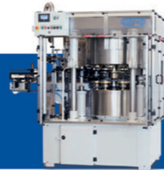
LINER/VERTICAL OVEN GROUP
