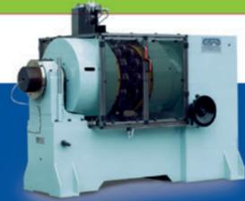
SCROLL SHEAR UNIT WITH SHEET FEEDER
